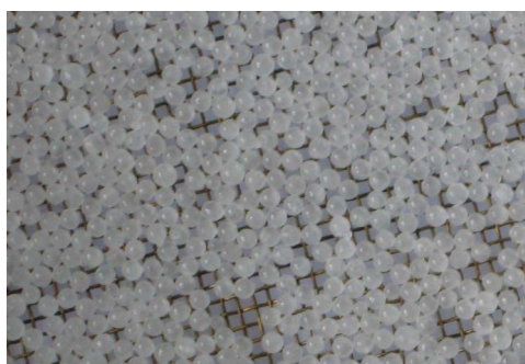
Figure 5. Light micrograph of PEG pellets by vibration and stirring.
